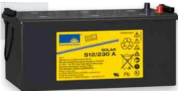
This is a heavy large specially made solar battery based on Gel design. This contains gel and no liquids and can be operated in any position. Weight is 73.5 Kg. Compared to car battery this will live about 10 X longer if deep cycled as here and if used in a warm area. When area is hot we add a fan cooler to get longer lifetime if temperature is over 30C when charged.
