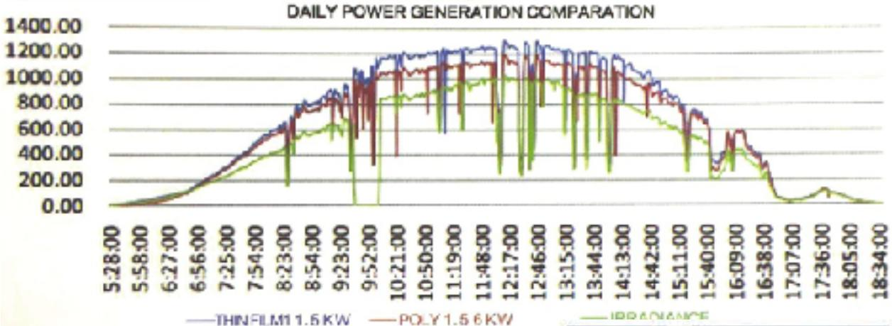
**Comparison** between Polycrystalline panels and a Si Solar panels a typical day side by side. Here it is clear the thin film is better all time. Drop outs here are passing clouds that shadow panels.
