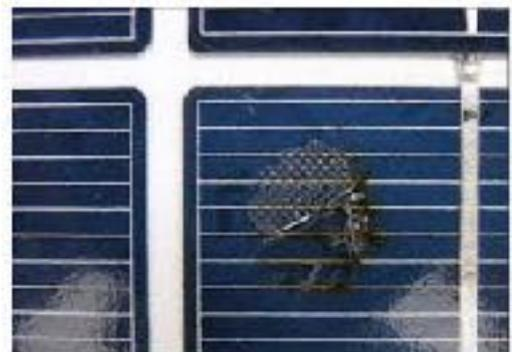
Image of solar panel shadow overheat and burned surface due to resistance change
