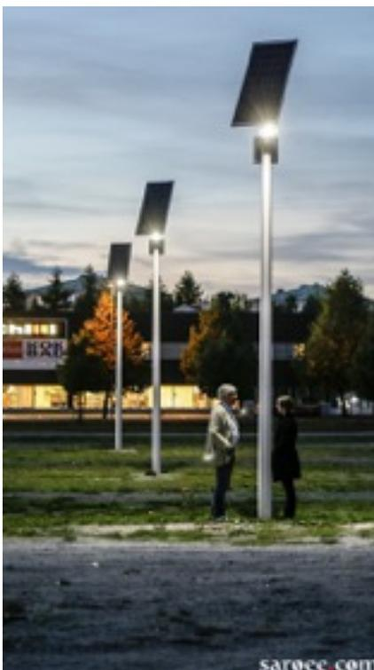
Solar street lamps have a solar panel + battery + electronics to operate for many years with no service and maintenance. We have many systems used in Kenya for 5 years with no service demands. Battery is an advanced lithium battery that can be charged at 60C and operate for over 5000 cycles. We have several sizes from 8 MW forecourt yard lamps to large solar street lamps of
