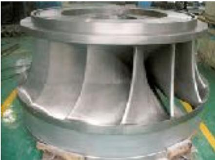
**Francis turbines** is the universal high end turbine. Water head starts at 10 meter and ends up to over 100 meters. Power range from 20 KW to several MW size. These turbines are good to handle large variations in flow with high efficiency. There are horisontal shaft and vertical shaft models.
