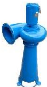
**Tube connected Kaplan turbines** are a bit similar but have a conn section by tube for incoming water and a draught tube as exit. They are a bit larger and starts at 1 KW up to 15KW output. Water head 4 meter to 15 meter.
