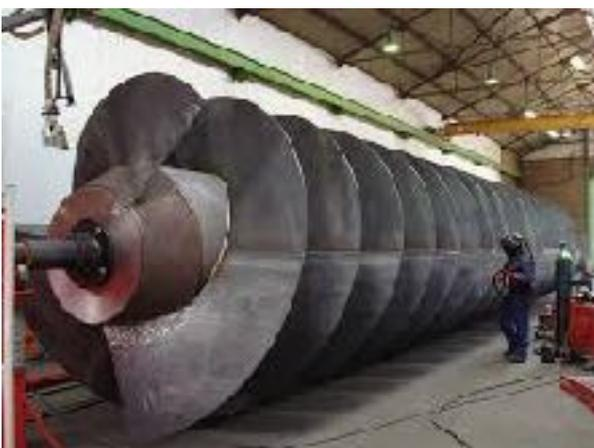
**Archimedes screw turbines** where water head is very low. Here we can get power from 1 meter watershed up to 5 meters. Power from a few KW to 100 KW. They are large and costly but often the only solution that can be used.
