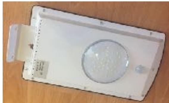
2016/2017 we have installed a number of Solar court yard lamps in Panzi Hospital in Congo and the orphanage in Lwala in Kenya. All have an integrated solar panel and a Lithium battery to supply the 12 W led lamp.
