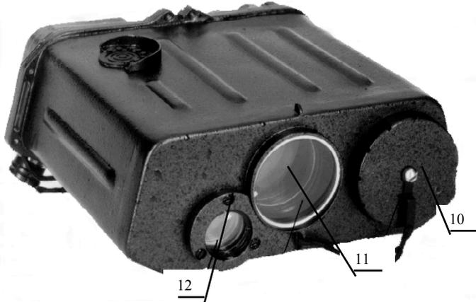
1 – trigger; 2 – **MODE** operating mode switch; 3 – desiccator with silica gel; 4 - plug to output information on range; 5 -boresight eyepiece; 6– digital display ocular; 7 - **ON** supply switch; 8 – external power supply and remote trigger plug; 9 – **MIN RANGE** minimum range (gate) handle ; 10 - battery compartment lid; 11 – receiving and sighting channel objective; 12– transmitting channel objective.
