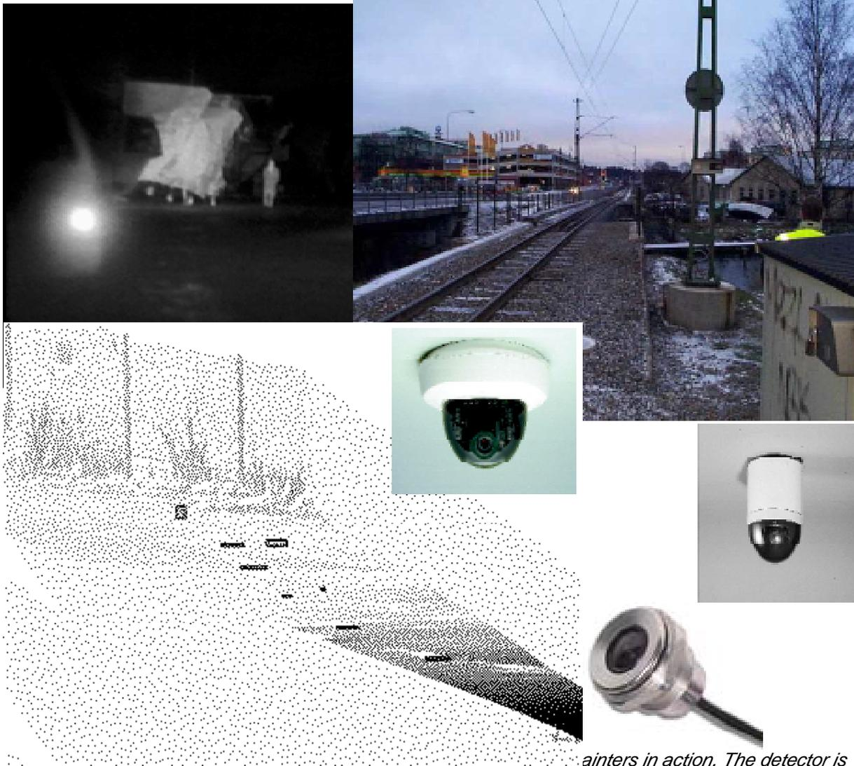
Painters in action. The detector is designed to cover wall and floor areas and when something is here it gives an alarm and starts up a video recording / camera system.
