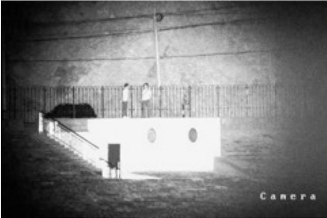
Man at a pier at 1500 meter in distance. Here we have an overview with not full zoom. It is night and very dark and the more bright area is the laser beam illumination. Here beam is slightly smaller than the field of view but this can be adjusted manually or be auto tracking.
