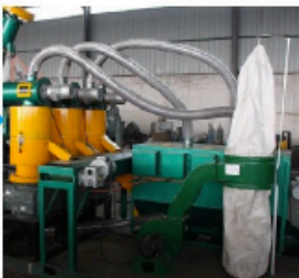
Cooler & Bag Dust Filter
