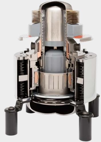
Thermal energy in the form of heat is fed into the engine. This thermal energy makes the helium in the engine expand, subsequently driving the piston. By cooling the helium it shrinks which causes the piston to move back again. The oscillating mechanical movement is converted into electrical energy by a linear alternator in the engine.
